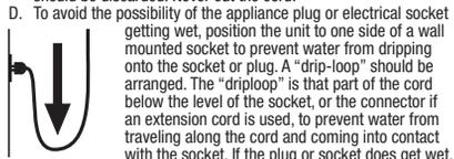
DO NOT unplug the cord. Disconnect the fuse or circuit breaker that supplies power to the appliance. Then unplug and examine for the presence of water in the socket.
