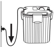
adjuster or adjust the height of the mounting bracket in order to hang the unit in a vertical position. It is very important to the proper operation of the filter that it be positioned vertically.
